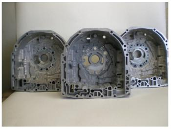
Fig. 5. Surfaces of collector cover at different stages of recovery
