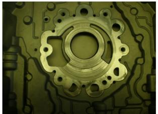
Fig. 4. Seats of leakage failure
